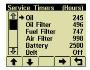
Pressing Button 4 • allows adjusting the selected service timer.
