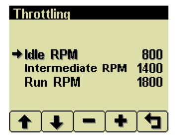
The throttling menu allows programming the automatic start/stop throttle profiles as shown in the following diagram.
