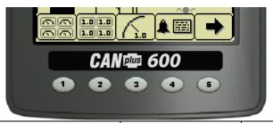
Five buttons access a context dependent **button bar** when any button from 1 to 4 is pressed. The graphical menu structure uses easily understood icons to indicate the button's current function. After 5 seconds of inactivity the button bar disappears.
