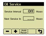
Button 1 — decreases the service interval time while Button 2 • increases the service interval time in 10 hour increments. Holding Button 3 for approximately 3 seconds resets Next Service In to the current service interval. The service timer descriptions can be changed using the CANplus Configurator.
