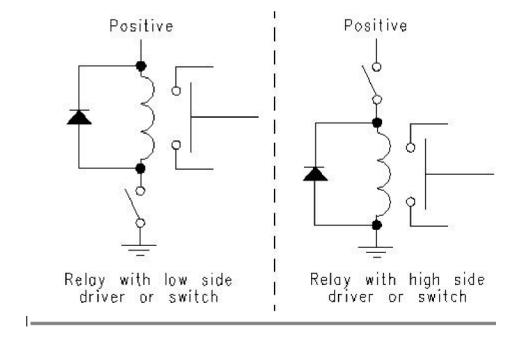
Relays and solenoids with built-in voltage transient suppression diodes are recommended whenever possible. Refer to the illustration for proper installation of diodes when built-in voltage transient suppression is not available.
