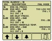
Example alarm message, alarm list screens showing unacknowledged conditions and acknowledged alarms.
