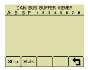
Button 1 stop freezes the display while button 2 states shows CANbus data statistics screen.
